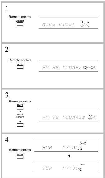
This unit features "ACCUCLOCK"-an automatic clock adjusting feature using RDS broadcast signals.
